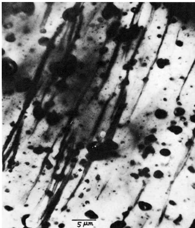
Fig. 7. Typical EPDM rubber-pp morphology and its relationship with crazing.
